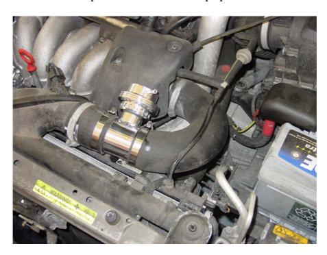
2/ Remove the air box lid as shown below in order to gain access to the original diverter valve located in the side of the turbo housing.
