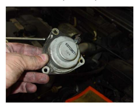
3/ Fit the vacuum pipe plastic joiner (supplied in the kit) to the open end of the original vacuum pipe, cut to length the silicon vacuum tube supplied and route to the new Dump valve vacuum connection. Refit the air box lid and all pipe work.
