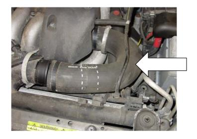
Mark the hose as shown. There must be at least 60mm of the hose sectioned off. We advise this to be done on the straightest part of the hose. Now cut the section out of the hose with a sharp knife. Fit the new T piece section and dump valve as indicated below. Tighten the T piece with the hose clips provided.
